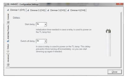
By using a start delay, the dimmer will only start dimming a few seconds after the power supply relay has been activated. This way the lamps have the time to start up first. The start delay can be set between 0 and 3 seconds.
