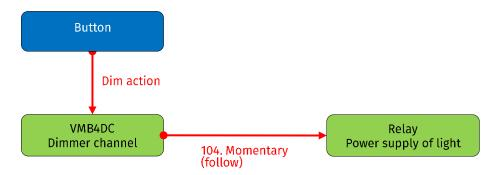
When the dimmer channel is set to 0%, the relay will be open. When the dimmer channel is set to a value different from 0%, the relay will be closed.
