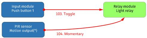
(\*) Set the on-time of the motion output channel in the configuration settings of the sensor module ("Timeout"), see also the FAQ and downloads of the sensor modules.
