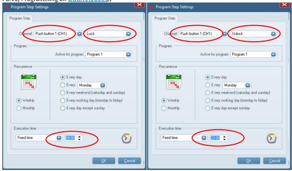
3. In the configuration settings of the sensor module, create program steps that lock the motion sensor at 22:00 and unlock it at 08:00.
