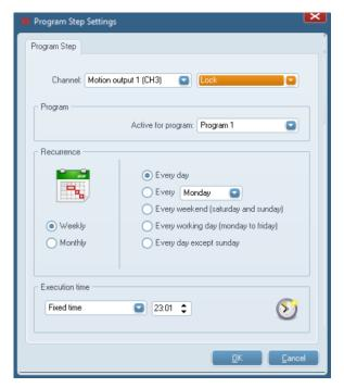
In the VMBPIRM or VMBPIRC configuration the timeout of the motion outputs is set to "Momentary".
