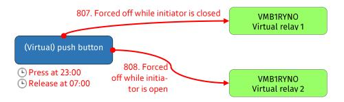
The (virtual) push button is activated by two program steps: press at 23:00 and release at 07:00.
