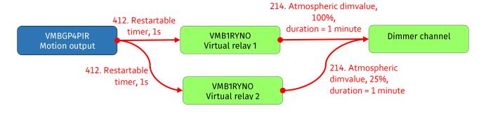
We then make sure only one dimming action can be active at any given moment. To do so, we use a (virtual) push button which forces the virtual relays off. Add the following actions and program steps:
