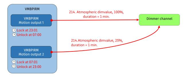
Motion output 1 is locked at night, and motion output 2 is locked by day, using 4 program steps:
